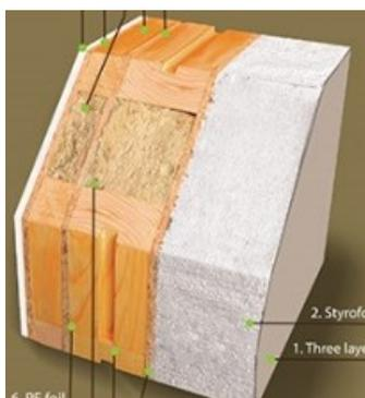
Figure 52: Conventional passive facade
