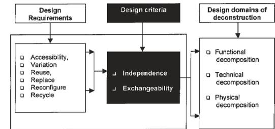
A structure can be reversed if its elements/component/systems are defined as independent parts of a building structure, and if their interfaces are designed for exchangeability. Independence of parts is determined primarily by functional design domains, which deal with design of material levels of technical composition of building and specification of independent material clusters.
