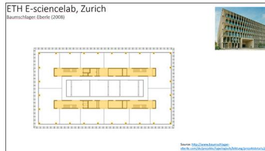
**Figure 26** Off-center clustered loadbearing, communication, installation core
