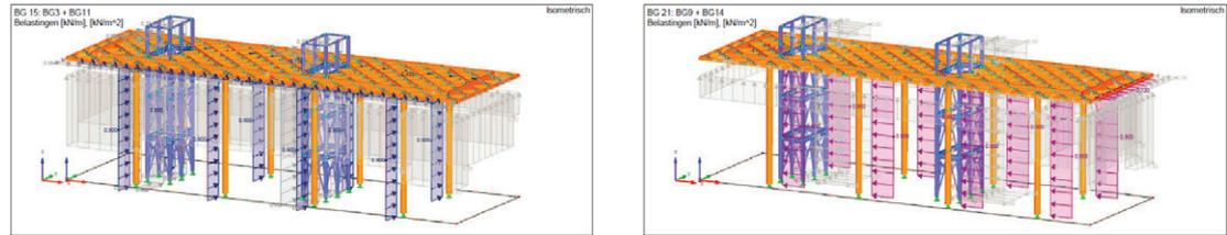
Figure 62 Analyses of impact of different load combinations on GTB Lab core elements
