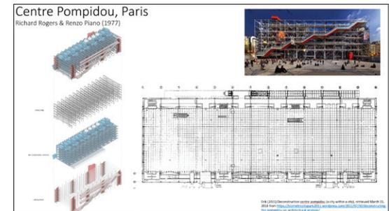
**Figure 30** Peripheral clustered loadbearing, communication, installation core
