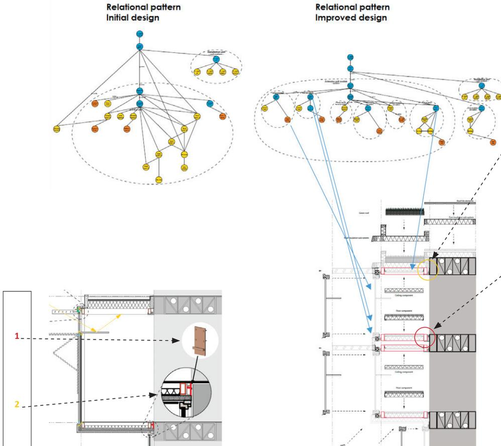
**Figure 45** Left the initial design of replaceable GTB Lab module involves assembly of all parts of the module on element level on the site. Right the improved design allows independent modifications disassembly of complete roof, floor and façade.
