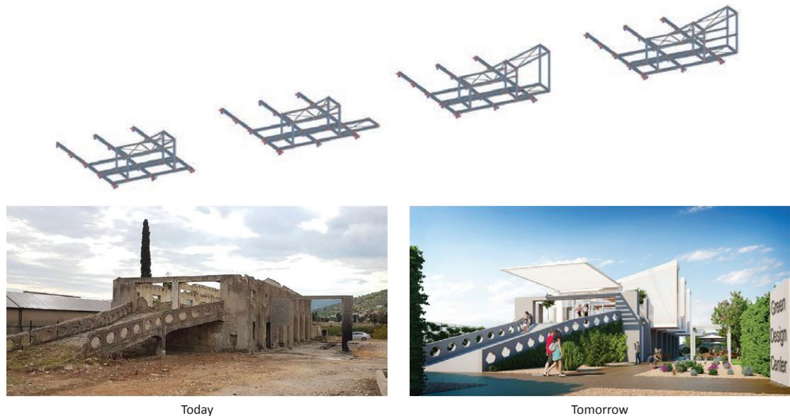
Figure 75 New steel frame as an intermediary between the old and the new part of the building structure and installation services.
