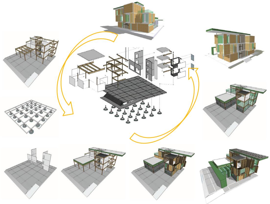
**Figure 2** Reversible Building with focus on high value recovery and reuse of building parts through design for reuse and reconfiguration. (Innovatie Catalogus 2017)
