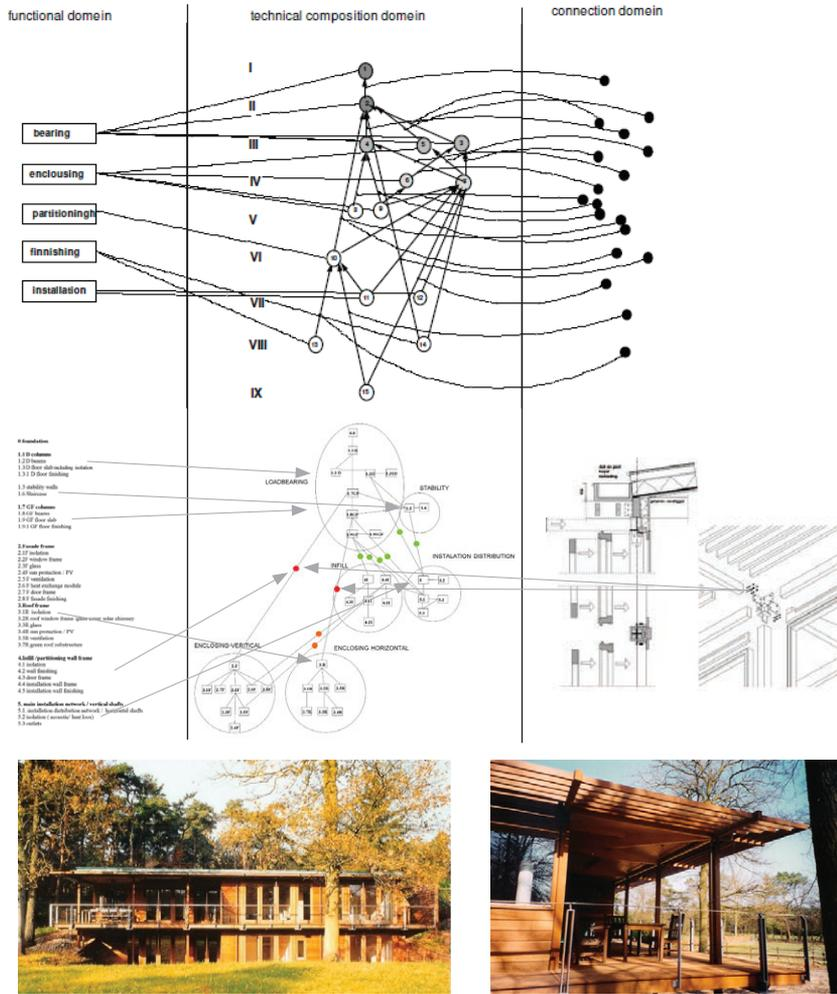
Figure 36 overview three key design considerations provisions of functional independence left by arrangement of building parts and group of part performing same function into an open hierarchy of parts and design of base elements and reversible connections which will guaranty physical independence of building parts (Design for Disassembly, Durmisevic 1999, 2016)
