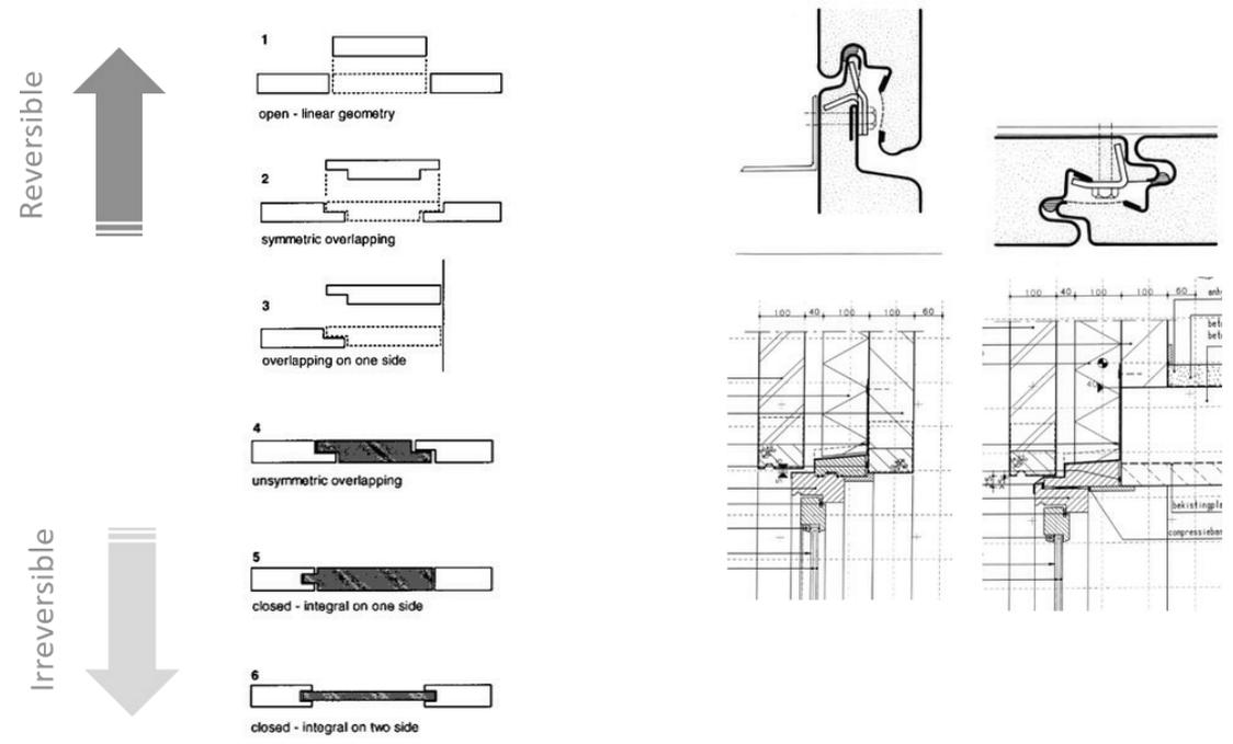
Figure 52 overview of principles geometries of product edge
