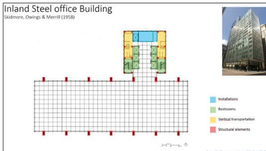
**Figure 25** Peripheral clustered loadbearing, communication, installation core
