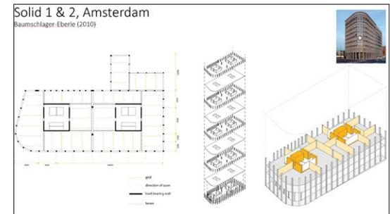
**Figure 27** Central clustered loadbearing, communication, installation core
