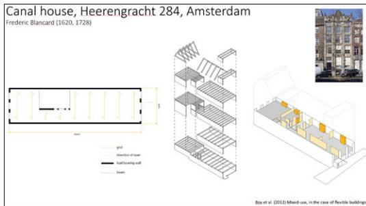
**Figure 28** Peripheral clustered loadbearing, communication, installation core ( Bos et al 2012)
