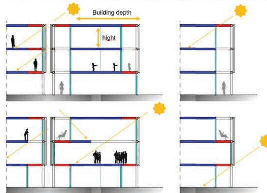
**Figure 22** Volume capacity analyses in relation to the building depth, height and typology.
