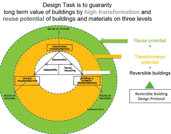
**Figure 4** three dimensions of transformation supported by reuse. Both reuse potential and transformation capacity are measures of the reversibility of a building. (Durmisevic 2006)
