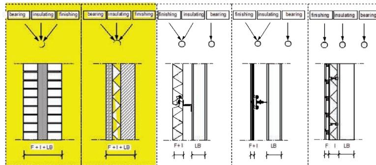
Figure 38 options representing functional independence/ dependency of the building exterior wall.
