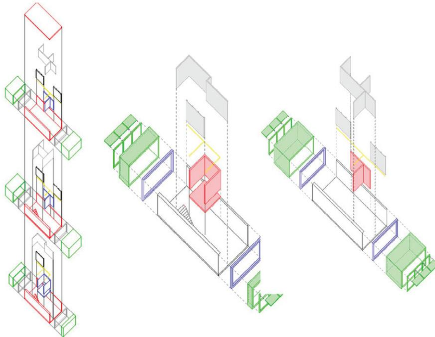
**Figure 34** Functional decomposition on building level: Wight surface represent existing permanent building structure; Red representing more permanent part (support, main technical services) of the structure but yet designed with the capacity to be disassembled at the end of the use life, green representing variable / exchangeable parts of the structure and blue representing intermediary between the permanent and variable parts of the structure while gray represent replaceable infill elements.
