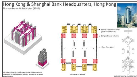
**Figure 29** Peripheral clustered loadbearing, communication, installation core
