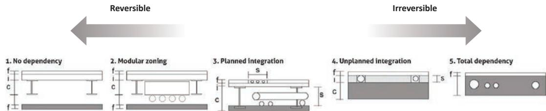
Figure 41 Schematic representation of five types of integration, the letters in the figure represent the following functions: (c) structure, (f) finish, (s) servicing and (i) insulation. (Durmisevic 2006)
