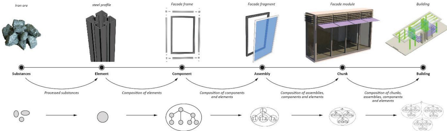
**Figure 43** Levels of assembly, aiming at assembly on bigger level of technical composition of the building
