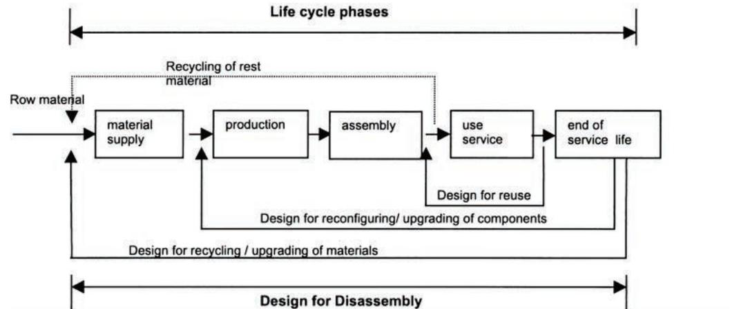
**Figure 1** Difference between linear model with focus on design for one end of life and circular model of material use in construction with focus on design for multiple life's and reuse options of materials (Durmisevic 2006)
