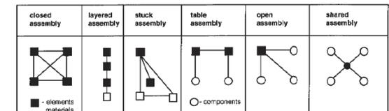
**Figure 46** Patterns representing five types of relations between building elements 1.closed assembly , 2.layered assembly, 3.stuck assembly, 4.table assembly 5.open assembly
