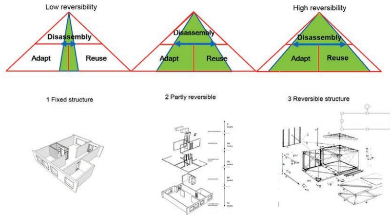
Figure 5 Key indicators forming a nucleus of reversible building design tools and protocol
