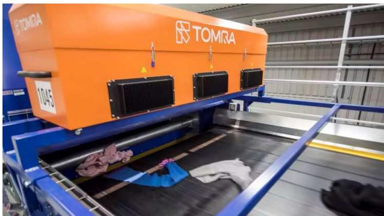
Figure 14: tri optique SIPTEX (source: Tomra)
