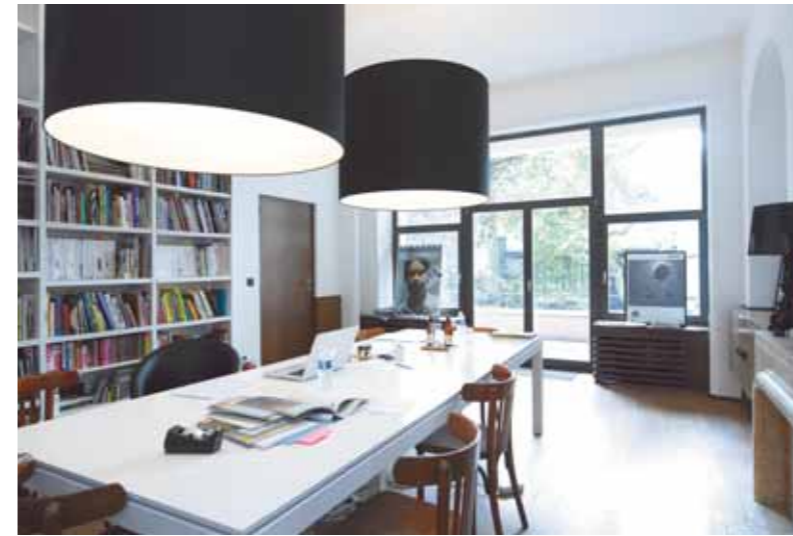
Renovation of offices on Rue Vanpé [014]: preserving the original façade, the architects chose to insulate the front from the inside. The old steel window frames have been preserved in the façade and new high-performance frames placed inside to ensure users' thermal and acoustic comfort (A2M architectes).
