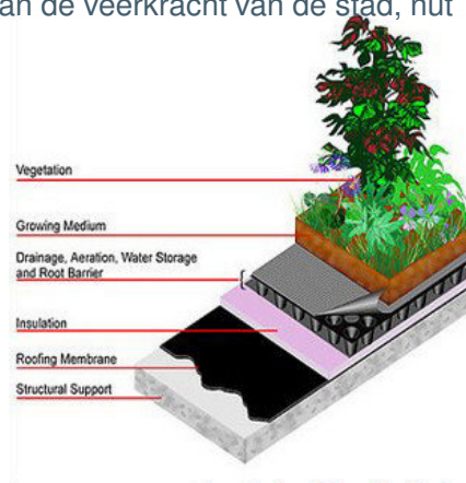
Cross-Section of Green Roof System
