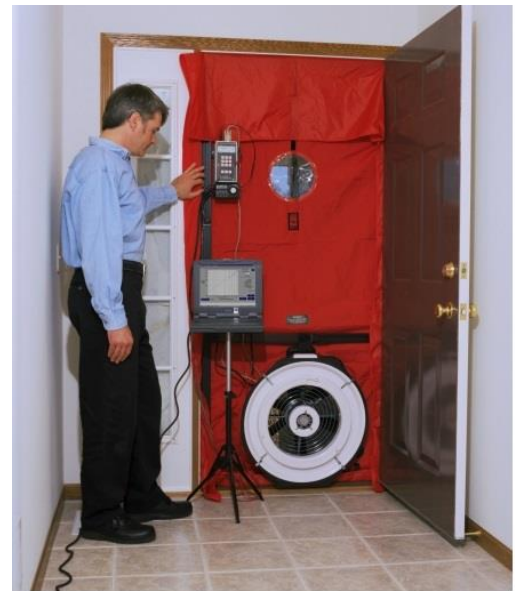
"Blower door" test
