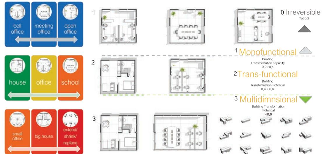
**Figure 20** Three Categories of transformable buildings with three levels of spatial reversibility
