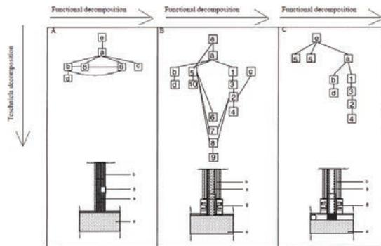
**Figure 50** Vertical relations represent relations within one functional group, while horizontal relations represent relations between different functional groups.
