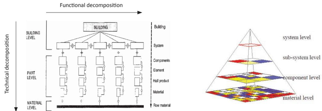
Figure 35 Hierarchy of levels of technical decomposition of reversible buildings (Durmisevic, 2006)
