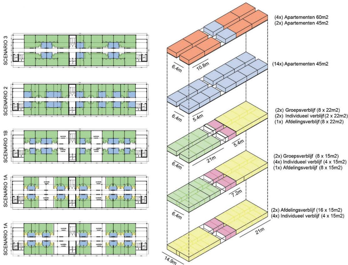
**Figure 11** Initial design phase/ feasibility study defining spatial reversibility and Transformation Capacity on building level indicating the compatibility of design solution with other desired use scenarios..
