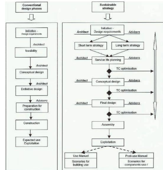
**Figure 8** left linear design approach right, RBD integrated design approach
