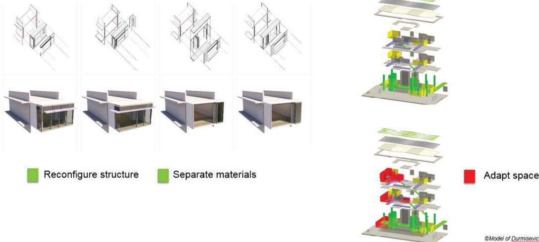
**Figure 19** Two categories of reversibility which address three design dimensions of reversible building design Spatial, structural and material (Durmisevic 2016)
