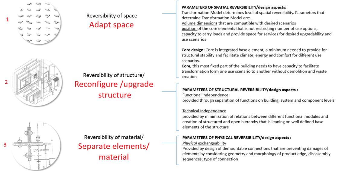
Figure 18 three dimensions of reversible buildings
