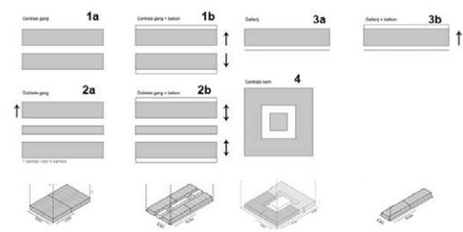
2. Typology in combination with the type and position of the core and clustering of fixed (core) elements, block dimension and distances between the cores
