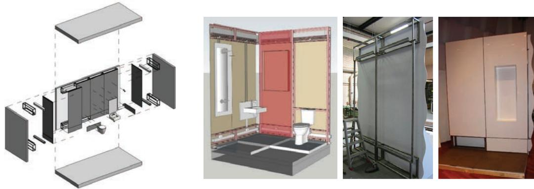
Figure 39 flexible building system defined by full separation of the main system functions (4D architects, Amsterdam 2009)
