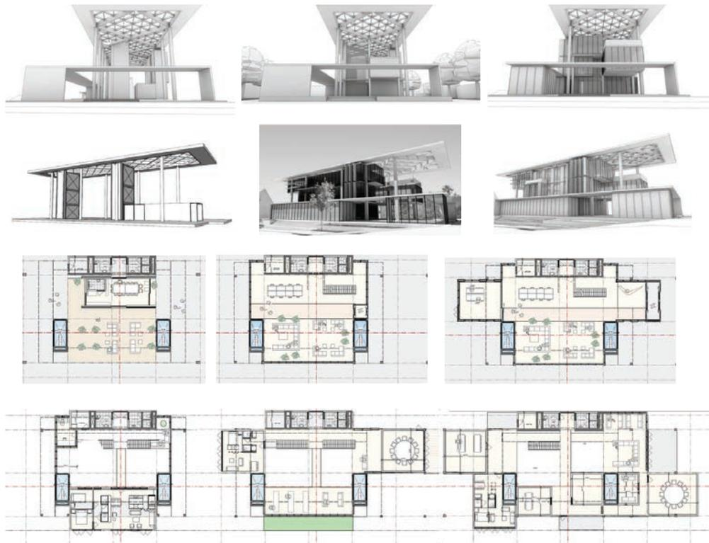
Figure 63 Possible reversible design scenarios in the Green Transformable Building Laboratory (GTB Lab)
