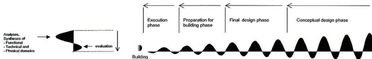
**Figure 10** design process as number of iterative decision-making loop containing analyses, syntheses and evaluation of design solution
