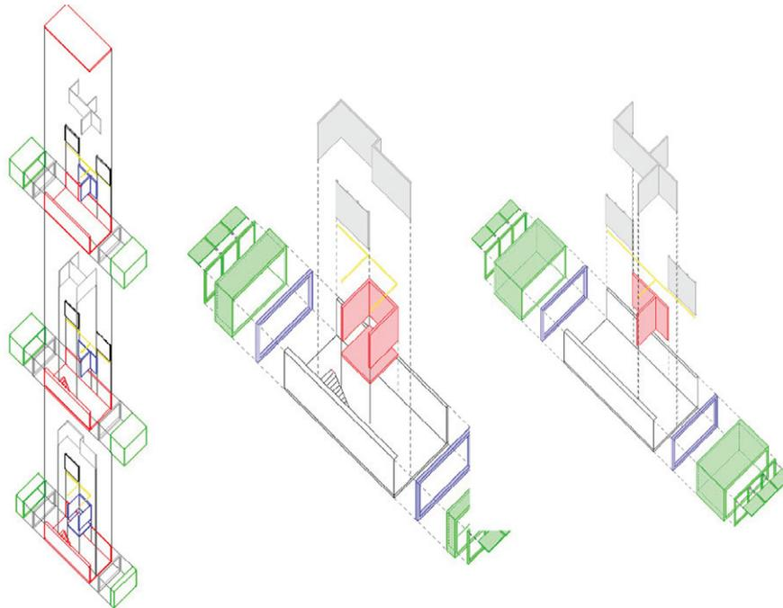
**Figure 34** Functional decomposition on building level: White surface represent existing permanent building structure; Red representing more permanent part (support, main technical services) of the structure but yet designed with the capacity to be disassembled at the end of the use life, green representing variable / exchangeable parts of the structure and blue representing intermediary between the permanent and variable parts of the structure while gray represent replaceable infill elements.
