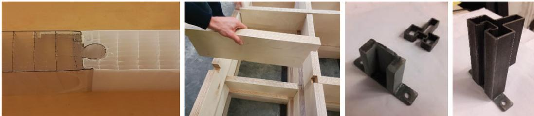
Figure 55 Examples of interlock connections.
