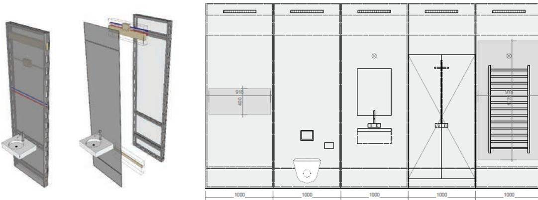
Figure 40 Flexible product made of elements representing individual functions. (4D architects, Amsterdam 2009)
