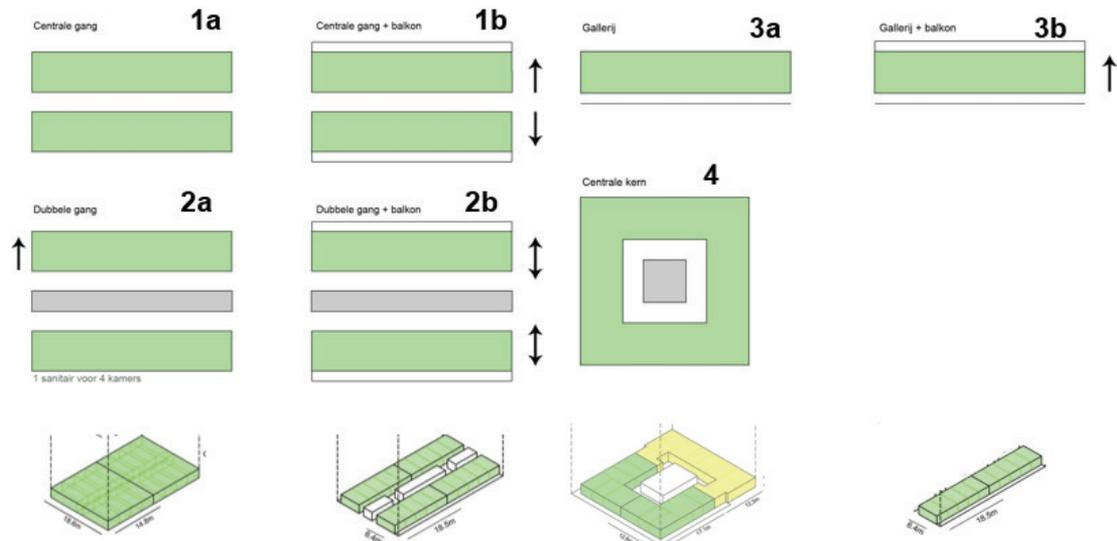
Figure 23 Four main building typologies
