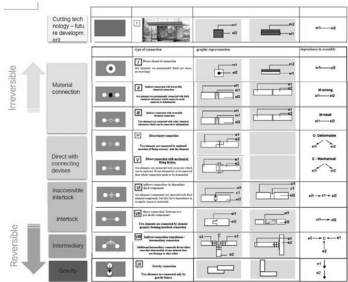
Figure 58 Ranking the connection types form reversible to irreversible
