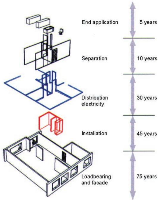
Figure 59 overview of hierarchy of type layers following the requirement of spatial flexibility within apartment
