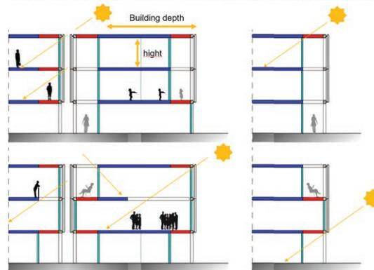
**Figure 22** Volume capacity analyses in relation to the building depth, height and typology.
