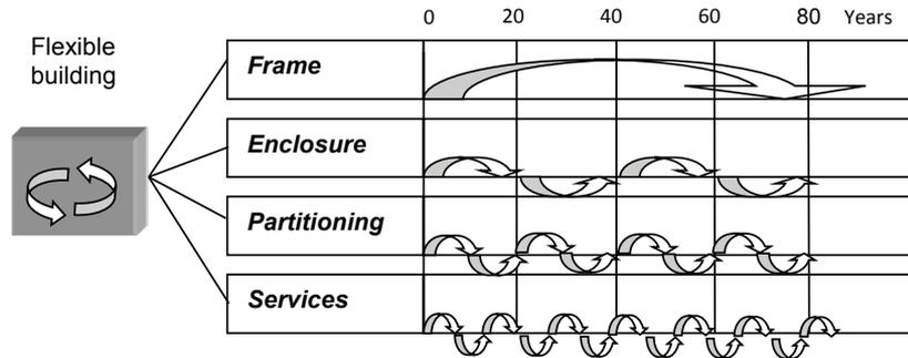
**Figure 3** Different durability rates of building components (Durmisevic 2006)
