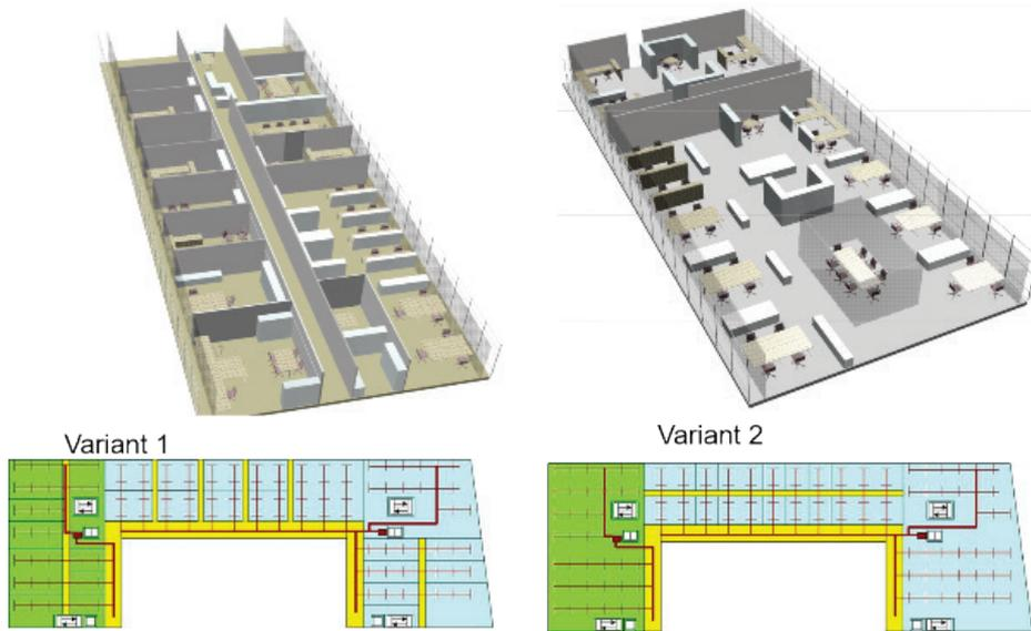
Figure 31 peripheral position of horizontal distribution of technical services enables different office typologies, 4D architects, Amsterdam 2003)
