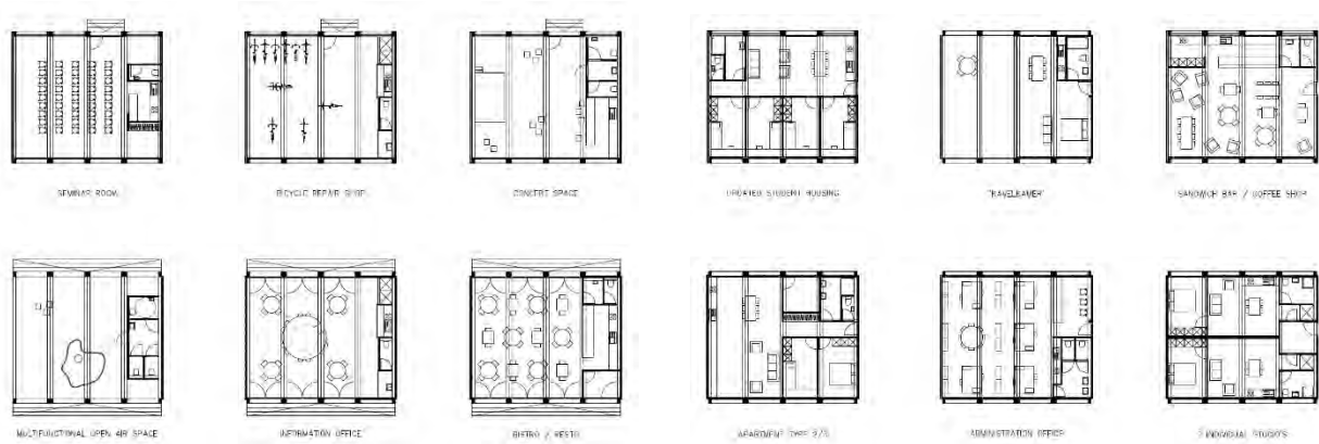
Figure 61: Analyzing the position of bathroom, kitchen and entrance within the different plan organizations drawn as research by design
