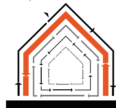
Figure 19: Stewart Brand's 'Shearing Layers' of a building
