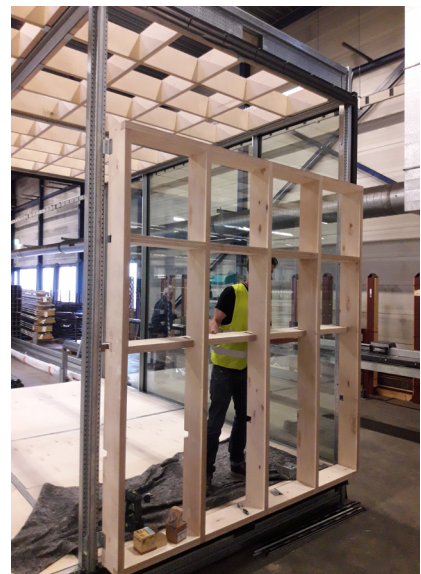
Assembling reversible triple glass panels with PV strips produced by Pilkington in Enschede NL.
