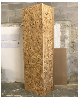
Figure 34: The insulated cassettes for the facade system were realised in the EFP workshop during the winter 2018
