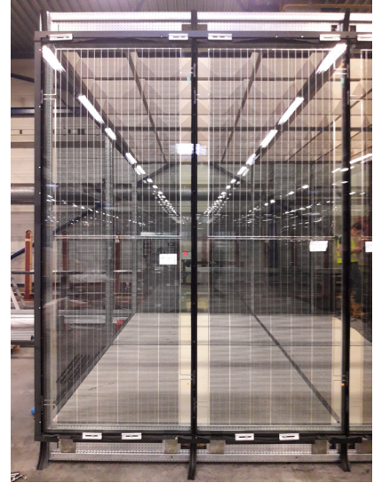
Assembling reversible triple glass panels with PV strips produced by Pilkington in Enschede NL.
