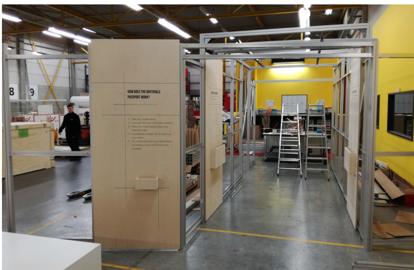
Uprights is placed and secured with wing nuts (two per upright)
