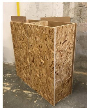
Figure 34: The insulated cassettes for the facade system were realised in the EFP workshop during the winter 2018
