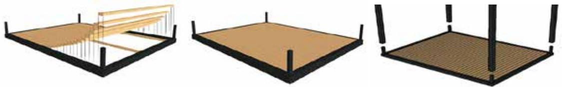
**Figure 108** Building up the ground floor
