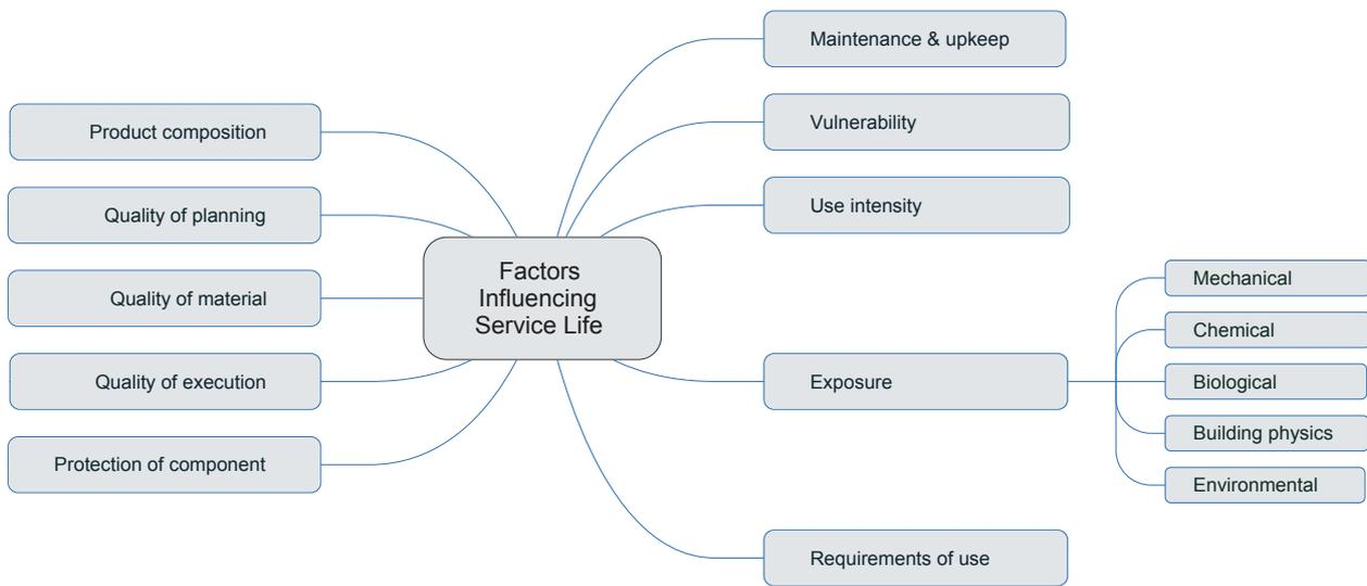
Figure 20: Selected factors influencing the Reference Service Life (RSL) of materials and products (Heinrich 2019b).
