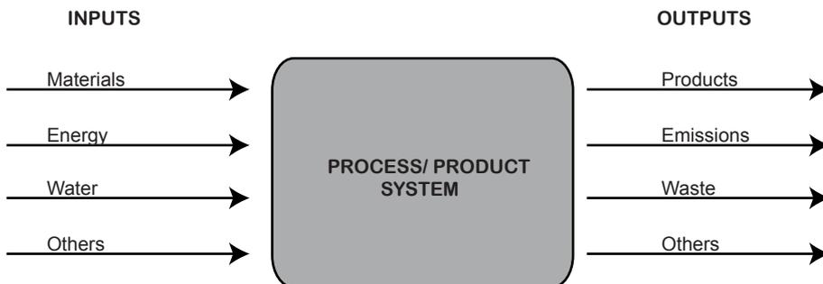
Figure 18: Material Flow Analysis (MFA)
