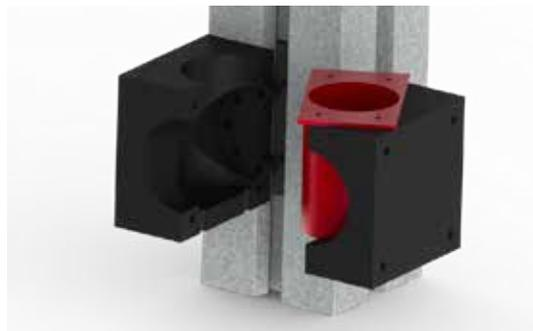
**Figure 112** Design of the hinges including all components, making rotations and replacement of components possible
