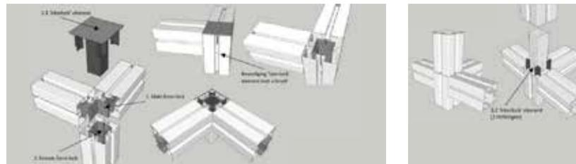
The interlock connection is made up out of three different base parts.
