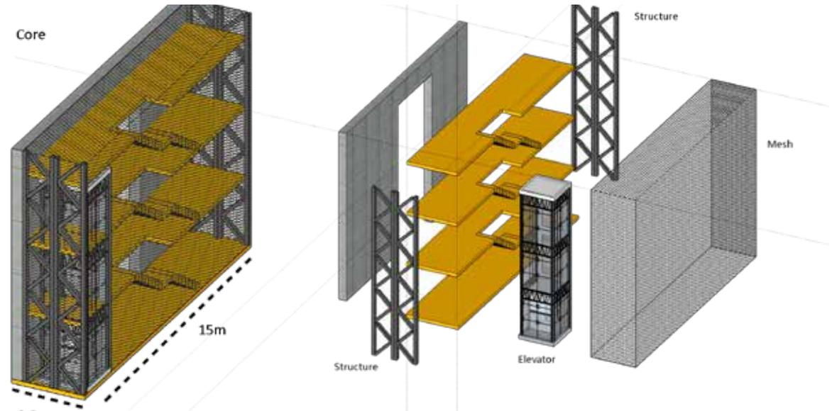
Figure 15 Exploded view core
