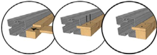
**Figure 109** Attachement wooden floor on the steel frame
