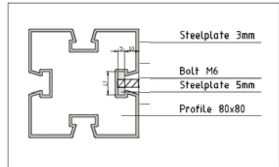
**Figure 113** Detail steel frame
