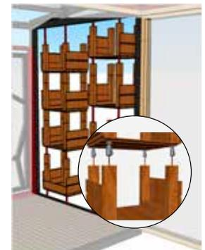
Figure 115 Creating a complete interior from existing wooden panels and beams based on boxes linked to each other or used separately
