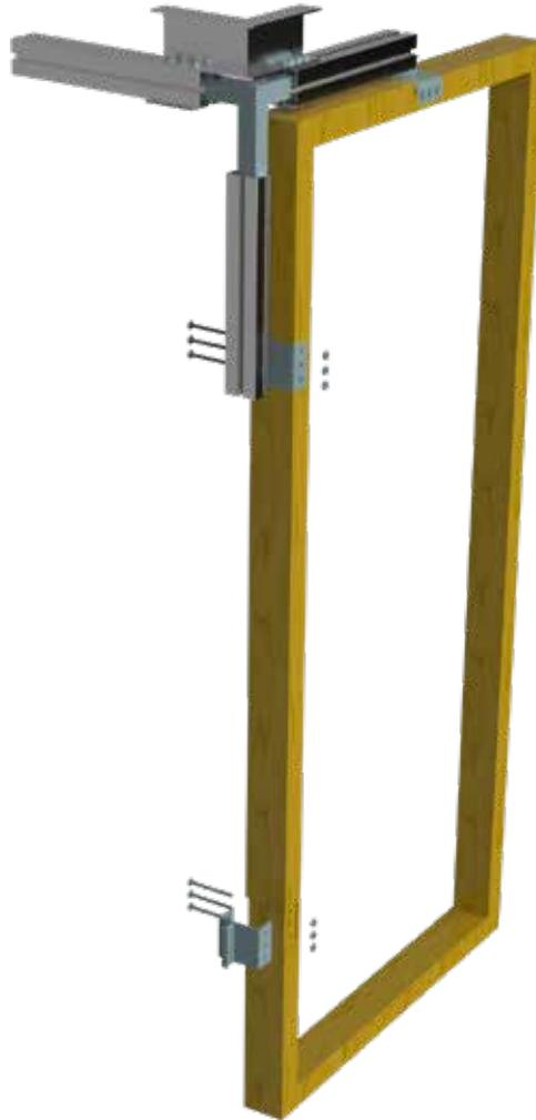
**Figure 138** Connection wooden frame - steel frame
