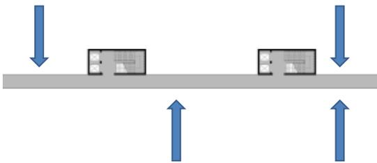
**Figure 25** Topview of the core showing the hallway and staircases. The blue arrows indicate how the modules can be connected.
