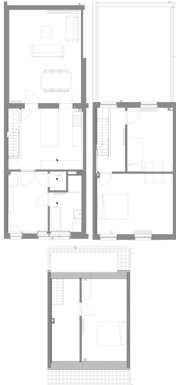
*Figure 7.9: terraced case-study , adapted for simulation (with added partition walls and doors between the originally open kitchen and the living area and stair well) (top: ground floor and 1<sup>st</sup> floor, bottom: 2<sup>nd</sup> floor) (copyright: BAST-architects & engineers)*
